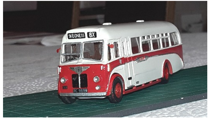
Trent's AEC Reliance with willowbrook body, Trent rebodied this bus in 1958 from B35F to FD39F
